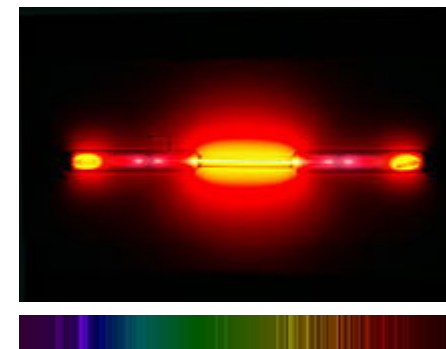
Spectral lines of neon in the visible region
